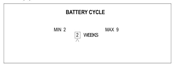
Figure 87 Set battery duration screen
